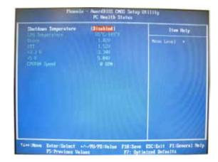
· Shutdown Temperature: selects the CPU temperature at which the system switches off.
