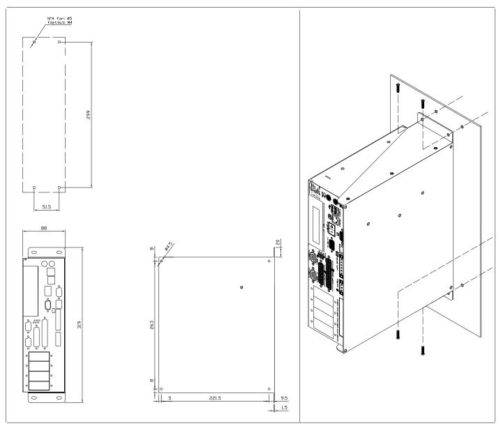
After having carried out the cuts on the plate as indicated in the template drawing, screw GF-BOX using the screws provided.
