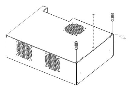
In order to open the rear cover insert the screwdriver into the slots A and B, apply some pressure in the direction indicated by the arrow.
